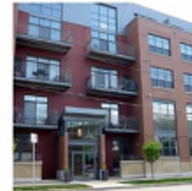
Where a building is visible from the street, locate the primary entrance on the front wall of the building, or where it will be highly visible.
